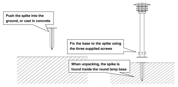
Alternatively use the supplied longer screws and plugs when fixing the base directly into the ground.
