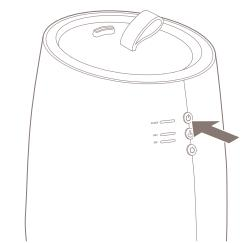
**Note:** If there is insufficient water in the tank when the device is turned on, the power/water supply indicator will turn from blue to red immediately. Please remove the water tank and refill it with water.
