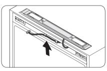
2. Move the connectors and wires to the opposite side. Insert the control cover, and then tighten the screws on the opposite side.
