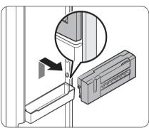
2. While holding the marked area on either side of the Slim Ice Maker unit with both hands, lift up the unit and pull out to the front.
