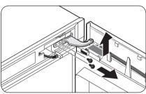
**4.** When the **top hinge** is removed, lift up to remove the freezer door. Keep the door in a safe place.
