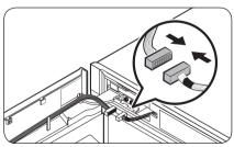
**7.** Connect the connectors from the freezer door and the main unit. Then, fix the wires on the inner hook of the optional hinge cover (L).
