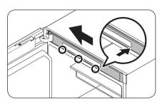
For models that have the display panel on the top of the freezer, push in the left end of the top frame cover then the right side by locking the lower and upper areas in this sequence.
