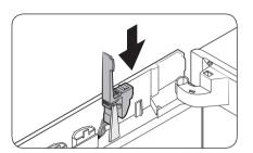
**6.** Reinsert the **dongle cover** in the original position.
