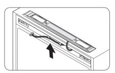
2. Move the connectors and wires to the opposite side. Insert the control cover, and then tighten the screws on the opposite side.
