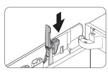
**6.** Reinsert the **dongle cover** in the original position.
