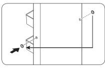
**3.** Use a flat-head screwdriver to remove the handle screw caps (x2). Then, insert the handle screw caps in the opposite side.
