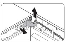
2. Pull out the left side of the hinge cover to remove, and then slightly lift up the bottom to pull out.
