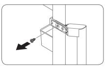
**2.** Remove each screw on the upper and lower side of the handle.
