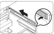
9. Insert the top frame cover with the part (b) fitting in the part (a) diagonally. Then, slide the end of the cover to the left to lock.
