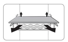
Slightly lift up the rear side of the shelf to pull out.
