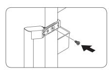
**1.** Insert the handle in the opposite side, and then tighten the screw.
