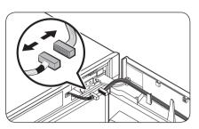
**3.** Disconnect the connectors on or around the freezer door. Loosen the screws from the **top hinge** to remove.
