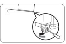
To adjust the height of the right side: Insert a flat-head screwdriver into the leveller of the front right leg. Turn the leveller clockwise to raise, or turn it counter clockwise to lower.
