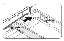
**9.** Insert the top frame cover with the part (b) fitting in the part (a) diagonally.
