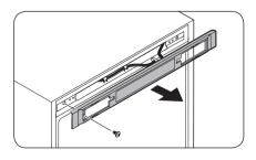
**1.** Remove the screw and pull out the control cover.
