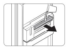
Pull up the handle of the water bin (01) to open, and then fill the bin with water up to the max line. Gently close the bin so that water does not drop or leak.
