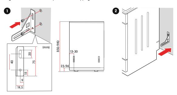
Fasten the bracket to the wall using the supplied screws and anchors.
