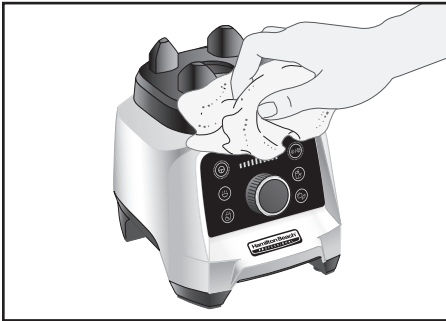
3. Wipe Blender base, control panel, and cord with a damp cloth or sponge. To remove stubborn spots, use a mild, nonabrasive cleanser.
