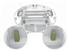
Wipe the inner and outer sensor ports on the bin with a clean, dry cloth.
