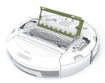
2 Remove the extractors and remove the yellow extractor caps. Remove any hair or debris that has collected underneath the caps and around the metal axles.
