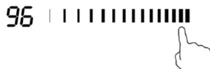
When the time is set, it will begin to count down immediately. The display will show the remaining time and the timer indicator will flash for 5 seconds.
