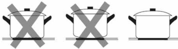
Make sure that the base of your pan is smooth, sits flat against the glass, and is the same size as the cooking zone. Use pans whose diameter is as large as the graphic of the zone selected. If you use a pot that is slightly wider, energy will be used at its maximum efficiency. If you use smaller pot, efficiency could be less than expected. Pots smaller than 140 mm may not be detected by the hob. Always centre your pan on the cooking zone.
