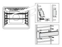
Click-on pull-out guides can be attached in any space between two wire guide levels. Place the guides symmetrically onto the wire guides on the left and right side of the oven cavity. First, hook the upper clip of the guide onto the wire of the wire guide. Then, press the lower clip into the right position until you hear a click.
