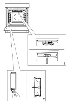
1 Unscrew and remove the cover (in anti-clockwise direction). Remove the halogen bulb.
