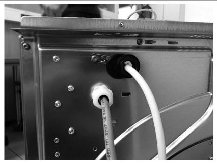
6. Where cable is routed through grommet, screw the grommet nut very tight, the cable pull out force of **>100N** and rotational force of **≥0,35Nm** without movement must be assured!
