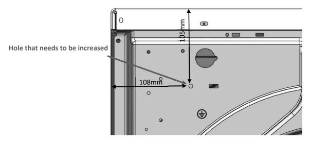
1. Diameter of hole which is marked on the picture needs to be increased from Ø5.5mm to Ø21mm.
