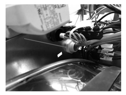
2. Install the cable through grommet as shown on picture above.
