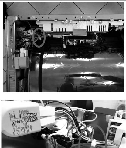
5. Route the cables as shown on picture above, use cable tie to hold the cables together.
