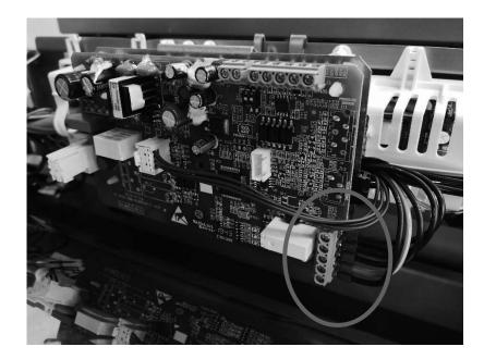
4. Connect the wires on relay board (EADBS).
