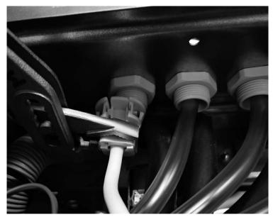
12. Use strain relief that was in the kit, mount it to the cable from inner side of washing machine right next to grommet, make sure no gap is left between grommet and strain relief. Squeeze strain relief tight with appropriate tool (pliers).
