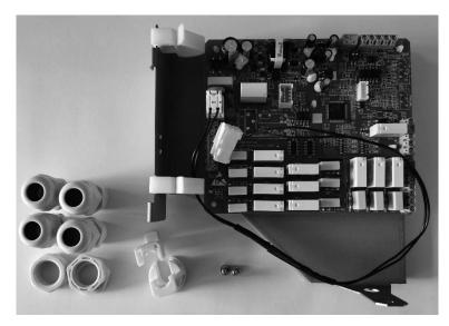
Kit includes: 4 grommets with nuts\*, EADBS board mounted on a bracket with wiring harness holders (2 pcs), 2 screws for fixating EADBS kit in WM, wiring harness for connecting power to EADBS (from input filter to EADBS) and strain relief for cable.
