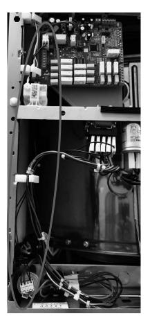
3. Route power supply wiring harness to rear side of washing machine, under electro component bracket and connect it to input filter as shown on picture above.
