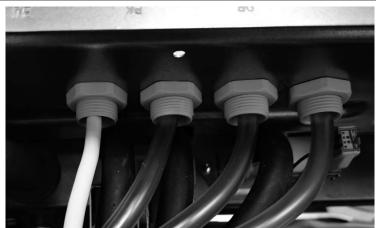
7. Install all the hoses and cable through grommets as shown on picture above.
