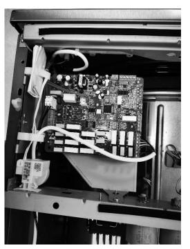
1. Install kit in washing machine on position as shown on picture above, route the harness that is in WM through cable holders (white plastic holders).
