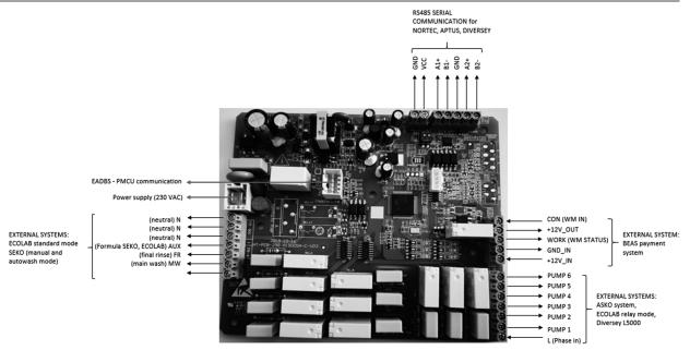
9. Connect your external system according to this electrical diagram.
