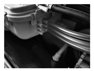
8. Drill the holes on detergent dispenser where the hoses will be connected with an appropriate size drill bit and then connect hoses as shown on picture above.
