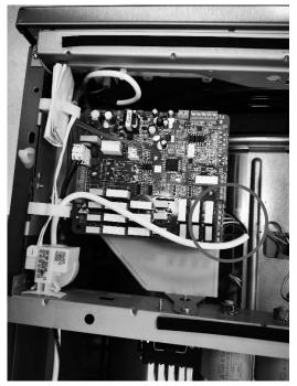
10. Connect the wires (cable) for external system to EADBS board terminal. On picture above is shown example of connection for external ASKO pumps. <u>When stripping the cable to expose wires, do not strip more than 50mm of cable jacket (see picture above).</u>
