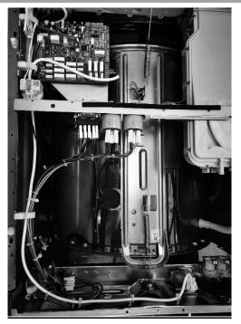
11. Route the cable for external system as shown on picture, use cable ties to fixate the cable to existing harness inside washing machine.
