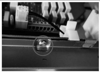
4. Using two screws that are part of kit, fixate EADBS holder to washing machine side panel and electro component bracket.
