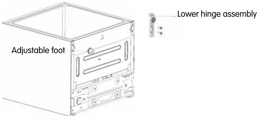
5) Install the lower hinge and adjustable foot on lower left side of the cabinet and lower right side respectively.
