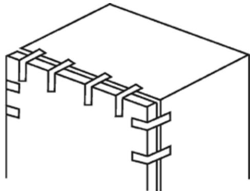
2) Remove the hole caps, the upper hinge cover and screws that secure the upper hinge, then remove the upper hinge. Make sure the door remains vertical during this process so that it does not fall over.
