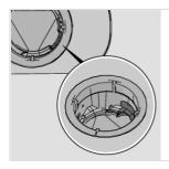
Check that the coloured stop on the right in the bottom drain is in place.
