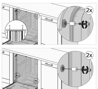
After fastening the machine, check that the front feet still touch the floor.
