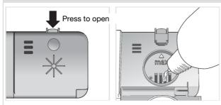
Add rinse aid to the container for rinse aid (if the dishwasher has not been connected to a system for the automated dosage of rinse aid).
