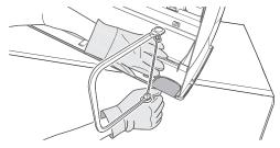
2 Remove any burrs along the cut section using a half round needle file.
