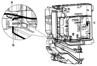
a S21 wire harness routing for wireless adapter
