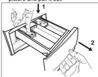
Remove the top part of the additive compartment to aid cleaning and flush it out under running warm water, to remove any traces of accumulated detergent. After cleaning, put the top part back into position.
