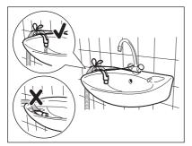
**1** Make sure that the plastic guide cannot move when the appliance drains and the drain hose end is not immersed in the water. There may be a return of dirty water into the appliance.
