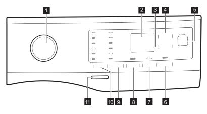
1 Programme dial 2 Display 6 3 Delay Start touch button 4 Flexitime touch button  $\bigcirc$  Night option □ 5 Start/Pause touch button 6 Easy Iron touch button = 7 Extra Rinse touch button 8 Stain touch button 😰
