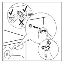
2. Position it toward left or right depending on the positon of the water tap. Make sure that the inlet hose is not in vertical position.
