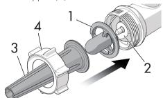
3. Insert the fastening ring nut (4) and screw it onto the body of the multi-food grinder, without overtightening.
