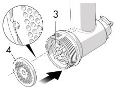
3. Screw the fastening ring nut (5) onto the multi-food grinder body, using the ring nut spanner if required, without overtightening.
