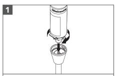
Insert the Blending Arm into the Motor Body and twist until it clicks to lock in place.
