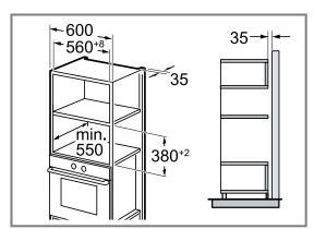
Do not fit the appliance too high up; it must be possible for accessories to be removed easily.
