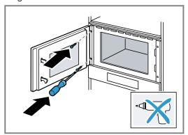
8. Remove any packaging material and adhesive film from the cooking compartment and the door.
