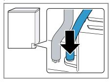
4. Insert the water drain hose into the hose guide.
