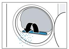
Ensure that no fluff falls into the air channel.
