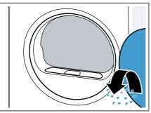
3. Remove the two-part fluff filter.
