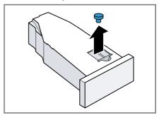
2. Insert the stopper on the underside.
