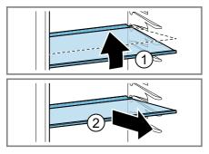
Press in the snap-in hooks on the side of the container ① and remove the front from the container in a turning motion ②.
