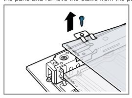
**6.** Remove the seal from below the pane. To do this, pull the seal and remove it upwards. Remove the pane.
