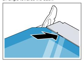
Ensure that the seal does not slip backwards.
