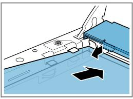
**3.** Fit the retaining clips onto the right- and left-hand side of the pane, aligning them so that the springs are over the screw holes. Screw the retaining clips in place.
