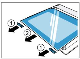
5. Unscrew the retaining clips on the right and left. Lift the pane and remove the claws from the pane.
