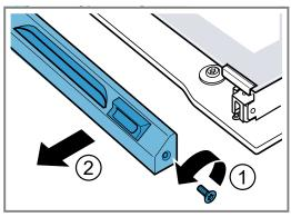
4. Remove the two small seals. Lift the top pane up and out.
