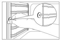
Pull the rear end of the shelf support away from the side wall and remove it.
